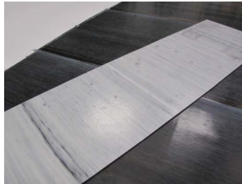
4-layered 90° laminat cut into specimen shape with an added TPE layer
