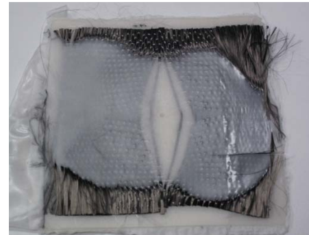
TPE/C-Fiber laminat after injection-moulding at 190°C into a cold cast
