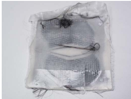
TPE/C-Fiber laminat after injection-moulding at 190°C into a cold cast
