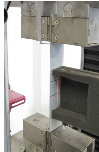
Optical strain measurement
