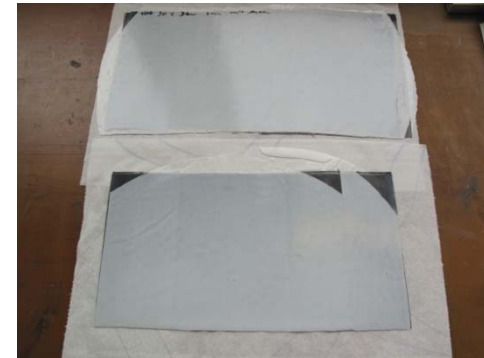
90°- specimen before cutting
